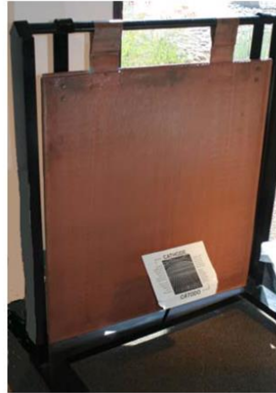
Figure 2. A copper cathode consists of 99.9% pure copper
