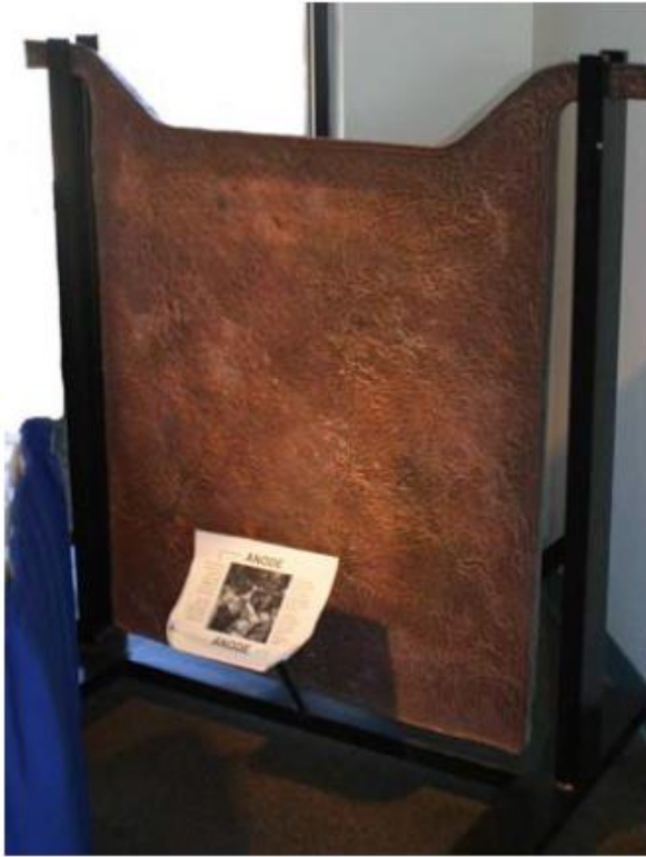
Figure 1. A copper anode consists of approximately 95% pure copper
